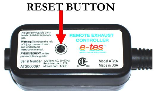
If you are using multiple E-TES SD units with multiple remotes, turn the other E-TES SD units OFF as you calibrate each remote to a specific E-TES SD to prevent signals from the other units from interrupting your calibration.
