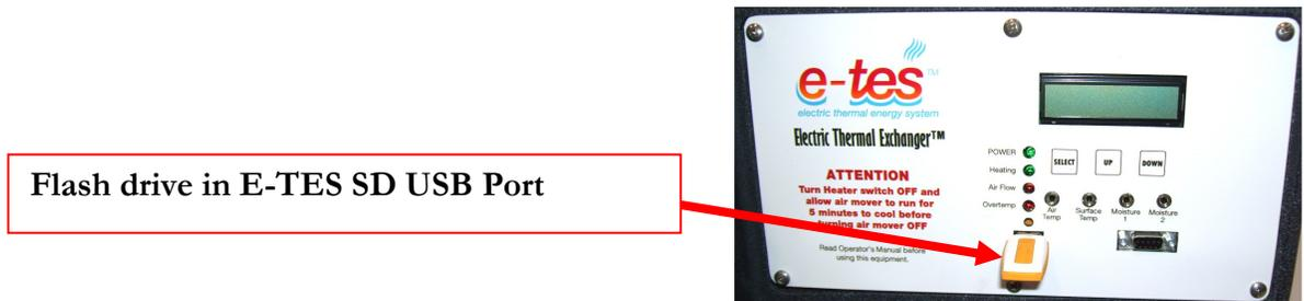
4. Press and hold both the UP button and DOWN button while you turn the power switch ON.
