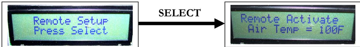
1. The Remote Exhaust Controller must be calibrated to work with the signal from a specific E-TES SD. To calibrate the Remote Exhaust Controller:
