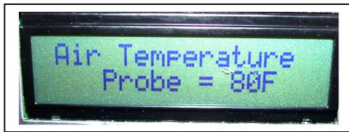
Press **SELECT** to set Air Temperature Probe shutdown temperature. Use **UP/DOWN** to change Air Temperature shutoff setting.
