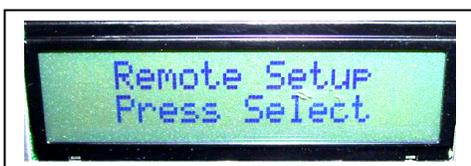
Press **SELECT** to set the E-TES Remote Exhaust Fan Control turn on temperature. Use **UP/DOWN** to change
