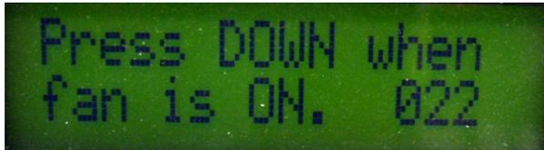
1. First turn the air mover OFF. When the fan is off and the number stops changing, press **DOWN**. This is the Off Set Point. (Shown as 000 in this example)
