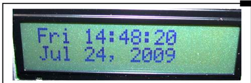
Press **SELECT** to set the E-TES SD Date & Time Clock. HOUR will flash first. Use the **UP/DOWN** buttons to change the HOUR setting. When correct, press **SELECT** to move to MINUTES, then SECONDS, MONTH, DAY NUMBER & finally YEAR. Use **UP/DOWN** to change each setting and **SELECT** to move to next option. When correct, press **SELECT** to save setting
