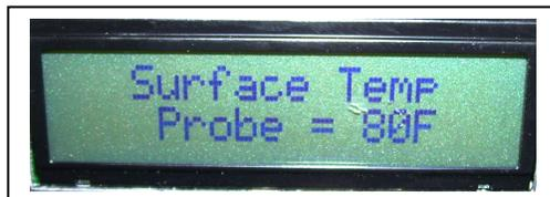
Press **SELECT** to set Surface Temperature Probe shutdown temperature. Use **UP/DOWN** to change Surface Temperature shutoff setting.
