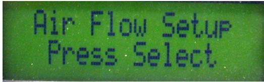
Press **SELECT** to set the Air Pressure Sensor trigger point. Follow the screen directions using the **DOWN** button to set the levels with the air mover OFF & ON.
